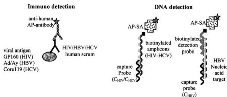
Fig. 2. Illustration of sandwich assays set up on CombOLISA for the detection of anti-viral antibodies (anti-HIV, anti-HBs, and anti-HCV) and viral nucleic acid targets (HIV, HBV, and HCV). HIV and HCV amplicons were biotinylated during amplification. HBV target was hybridized to a biotinylated detection probe. Alkaline phosphatase enzyme common to both assay formats allowed the simultaneous detection of nucleic acids and proteins.
