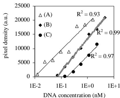
Fig. 4. Calibration curves for HBV (A), HIV (B), and HCV (C) nucleic acid targets assays carried out on CombOLISA. Pixel density measured on concerned spots is reported as a function of DNA concentration.
